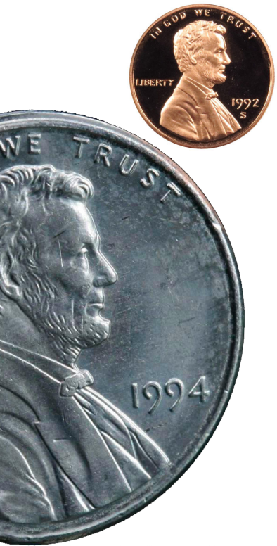
Pennies with copper surface removed. US pennies made after 1982 have a copper plating with a zinc core inside, a wildly used material yet not so easy to recycle.
